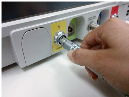
Figure 1-2 Connecting the N1923/4A cable to the 8990B peak power analyzer
